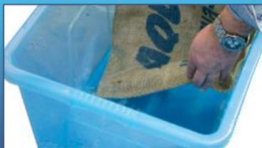
Immerse the bag completely in water for 5-6 minutes, to inflate them. For faster inflation, move the Bag around under the water and squeeze the material inside.
